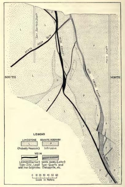
Fig. 59.—Cross-section through Tiro General shaft, Tiro General mine, Charcas, San Luis Potosi, Mexico. Shows two sets of veins. 1, The Leones type; sulphide veins, with blende, galena, and pyrite; first formed. 2, The Santa Isabel type, of quartz and chalcopyrite; formed later. At the bottom the two veins unite to form a compound vein (the Combination lode). By J. E. Spurr, 1911.
